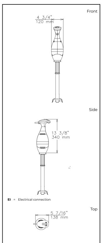
Electric Supply voltage: 110-120 V/1 ph/50/60 Hz **Total Watts:** 0.45 kW Plug type: USA NEMA 5-15P Key Information: External dimensions, Width: 5 7/16" (138 mm) External dimensions, 4 3/4" (120 mm) Depth: External dimensions, Height: 34 1/16" (865 mm) **Shipping width:** 11 7/16" (290 mm) Shipping depth: 27 3/16" (690 mm) Shipping height: 7 1/16" (180 mm) **Shipping weight:** 12 lbs (5.5 kg)
